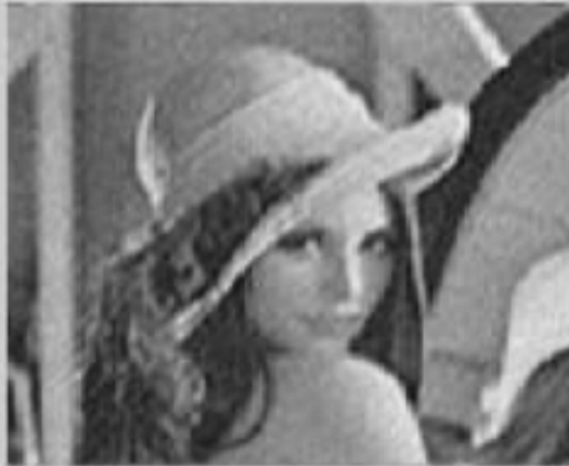
Fourier compression using 5% observation
